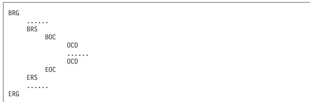
Figure 5. Structure of a resource group
